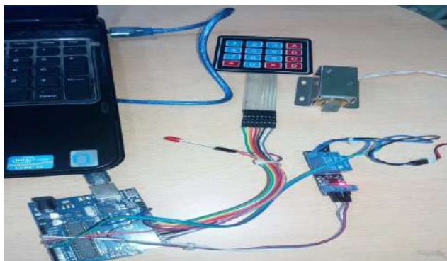
Figure (13) connection between Arduino, relay and solenoid.
